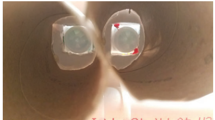
Figure 3: PIR Sensors Lenses with Physically Limited Sensing Radius
